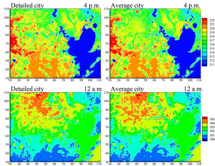
Figure 3. Average surface temperature (K) at 4 p.m. and 12 a.m. for the detailed and average city cases.
